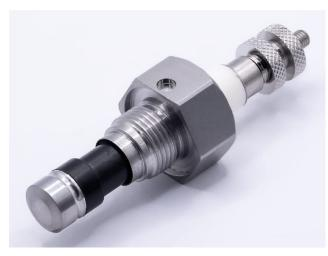
The Drumline DL459600802 is a direct replacement probe for the following OEM or aftermarket copies of the Hydrastep 459600802 electrode. Delta Mobrey has discontinued this electrode. The DL459600802 uses a superior design that consists of a brazed zirconia probe with a bearing grade PTFE coating.
